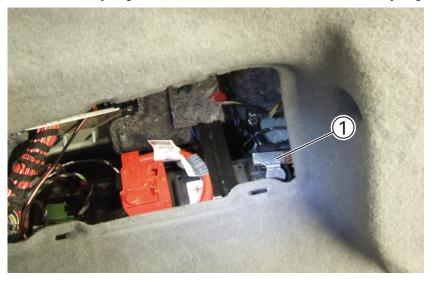
Fold up the luggage compartment floor lining (1). Release plastic nuts (2) and remove luggage compartment floor trim panel (1).
