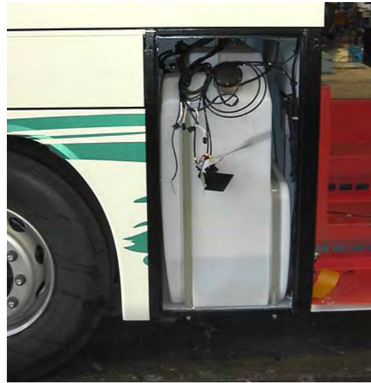
Figure 4: Coach - tank in the frame
