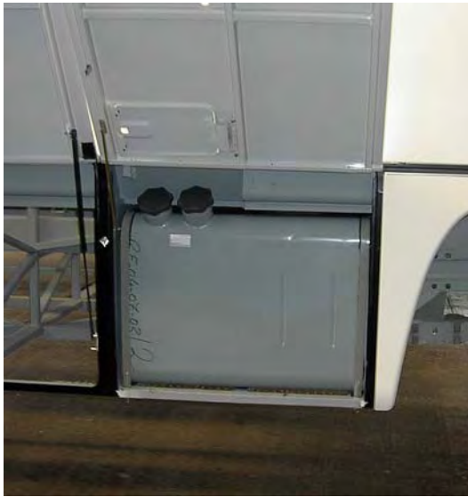
Figure 3: Interurban bus - tank in the body shell
