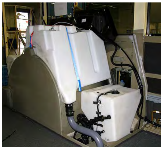
Figure 1: City bus - tank in the body shell
