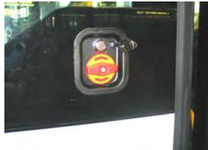
Figure 13: Outside emergency valve – example on city bus
