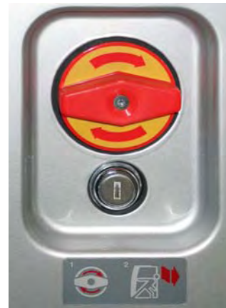
Figure 13: Outside emergency valve – example on city bus
