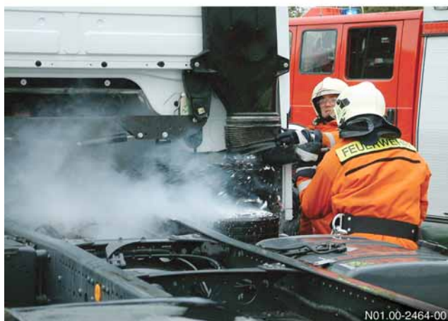
Blowing CO 2 into the air intake
