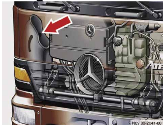
CO 2 injection point (arrow) at air intake
