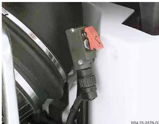
Possible location of EMERGENCY OFF switch on the right behind the cab
