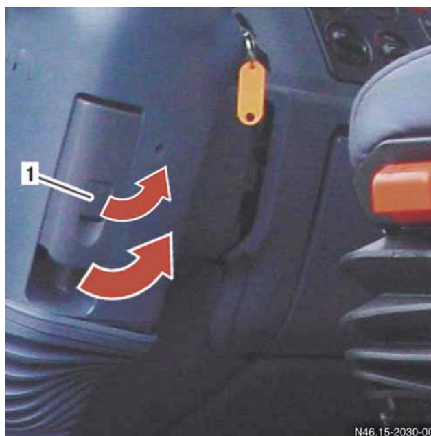
Manual release with locking mechanism
