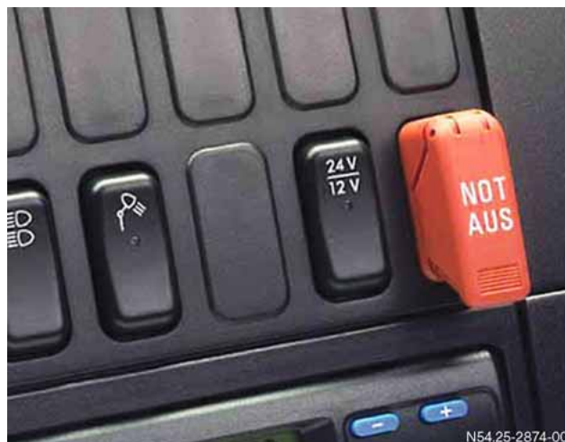
Location of EMERGENCY OFF switch in cockpit
