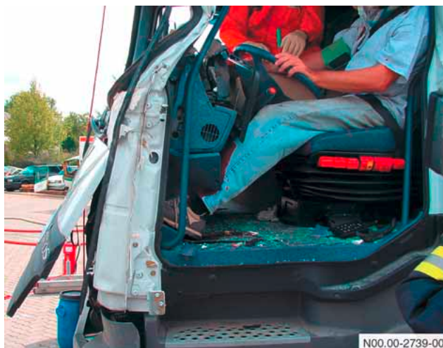
Deformed footwell (Rescue exercise at Ludwigshafen on 15.09.2001)
