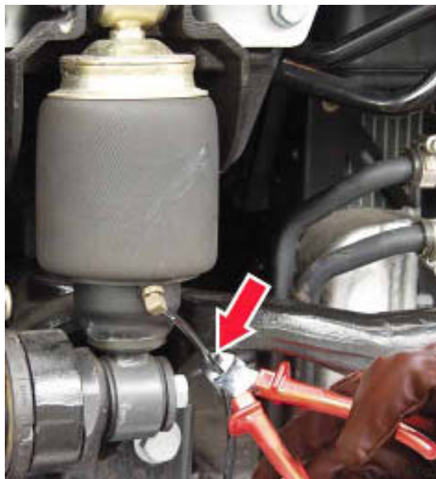
Cutting air line at air bellows
