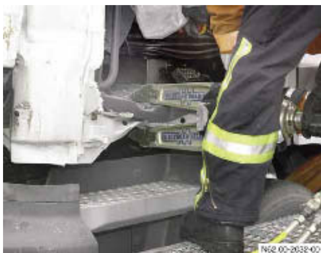
Crushing the rocker panel
