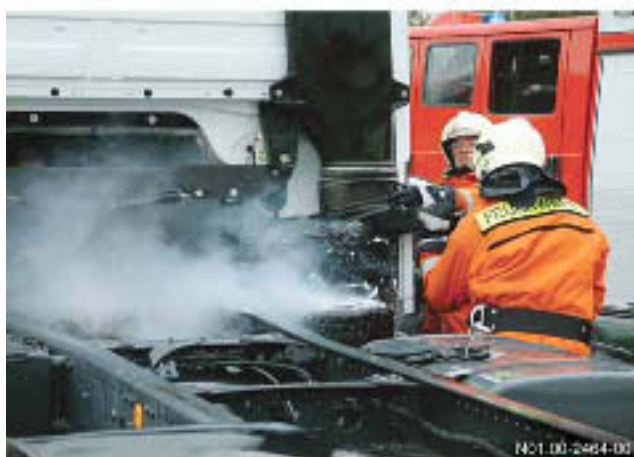
Blowing CO 2 into the air intake
