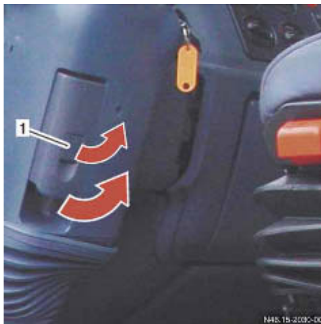
Manual release with locking mechanism
