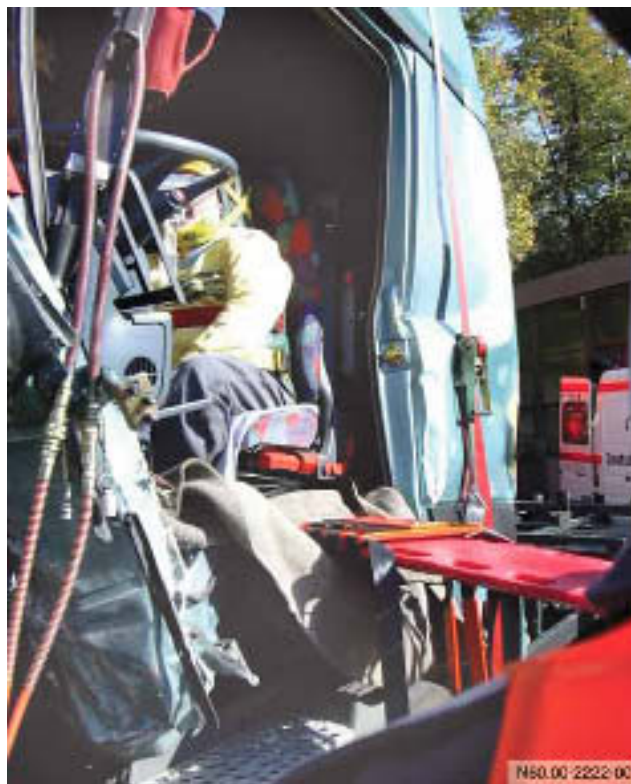
Rescue opening via the driver door
