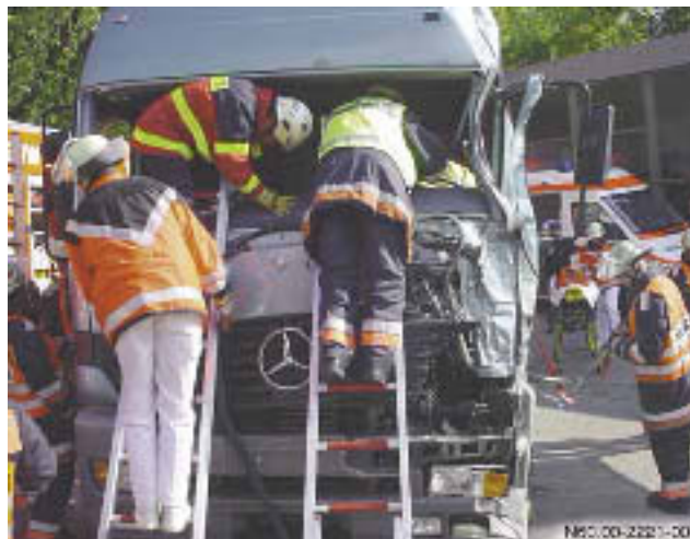
Access via a scaling ladder section
