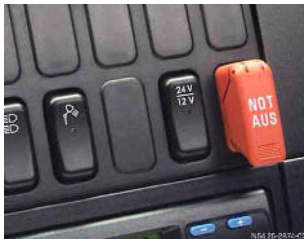
Location of EMERGENCY OFF switch in cockpit
