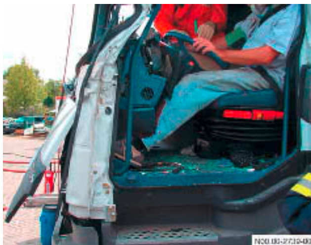
Deformed footwell (Rescue exercise at Ludwigshafen on 15.09.2001)
