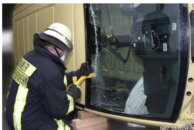
Sawing out a laminated safety glass windshield on a van that is lying on its side
