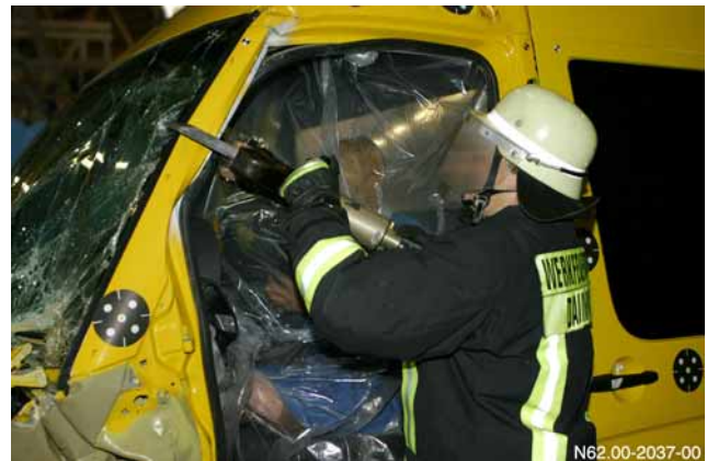
Cutting through the A-pillar at the height of the cutting mark
