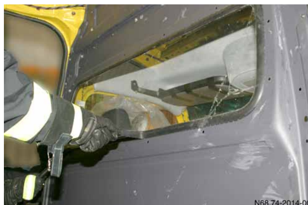
Glass management on partition wall window
