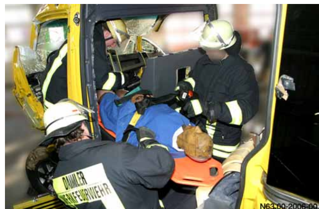
Rescue in the longitudinal direction, e.g. in MPVs or after removing the partition wall
