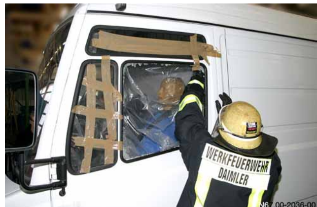
Procedure for removing a single-pane safety glass side window
