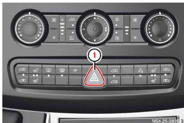
Hazard warning system switch
