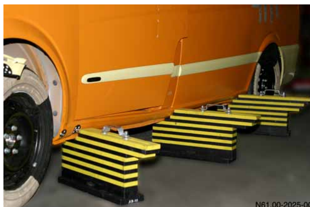
Supporting a van at 3 points on each side
