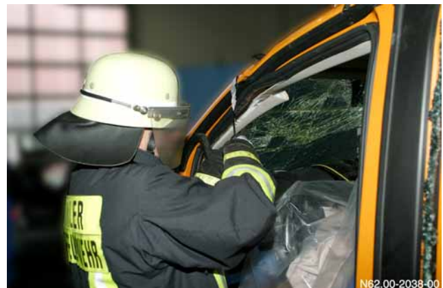
Removing the interior paneling Vito/Viano (model series 639)
