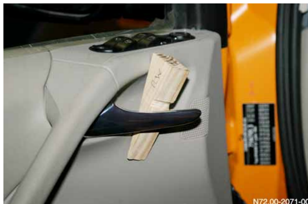
Inside/outside door handle held open with a wedge
