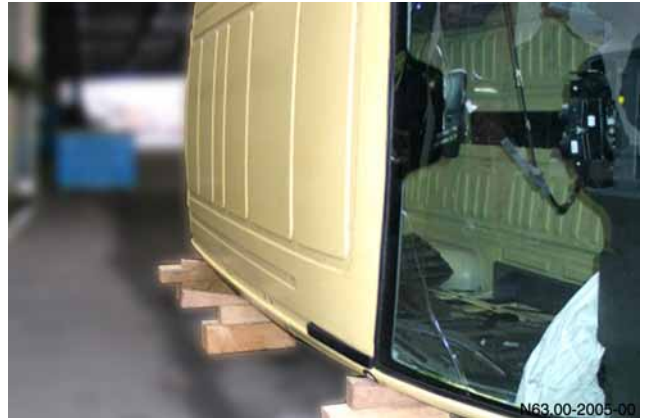
Securing a van lying on its side with wedges and blocks
