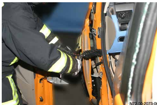
Cutting electrical lines with cable shears
