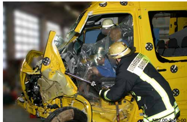
Using the telescopic rescue ram at the A-pillar
