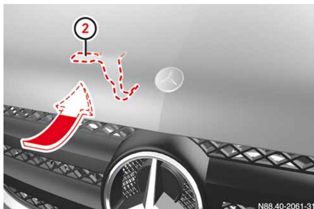
Opening the engine hood Sprinter (model series 906)
