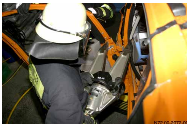
Forcing out the door at the hinges
