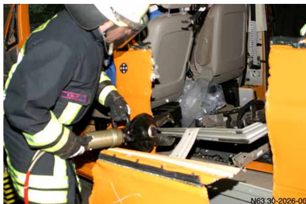
Bending down or removing the panel
