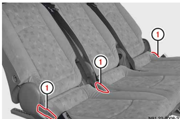
Tilting the backrest forwards
