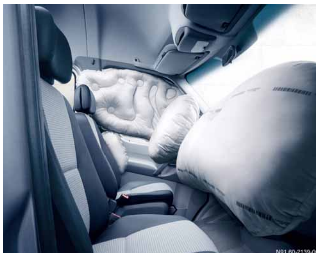
Location of the airbags Sprinter (model series 906)
