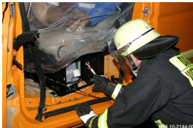
Disconnecting the battery under the driver seat in the Viano/Vito (model series 639)
