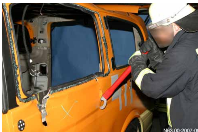
Making two cuts down to the level of the vehicle floor using a hooligan tool
