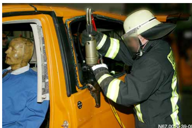
Cutting into the window sill on each side
