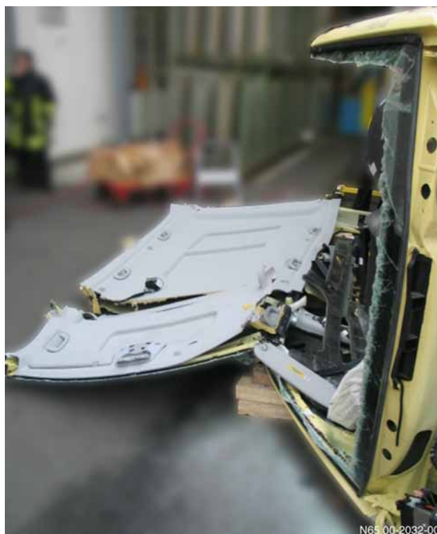
Roof bent down on a vehicle lying on its side
