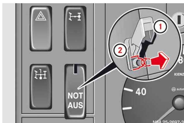
EMERGENCY OFF switch Vario (model series 667)
