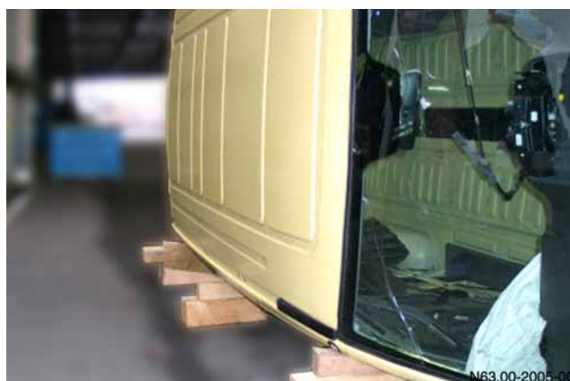
Securing a van lying on its side with wedges and blocks
