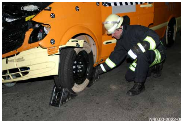
Using chocks to prevent the vehicle from rolling
