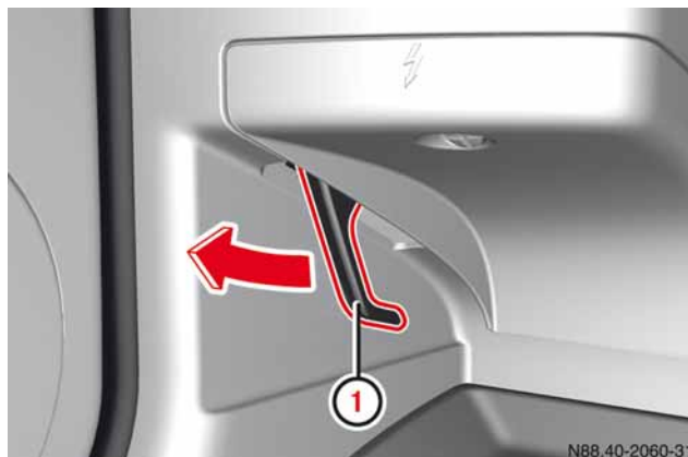
Opening the engine hood Sprinter (model series 906)
