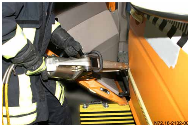
Removing a load compartment sliding door
