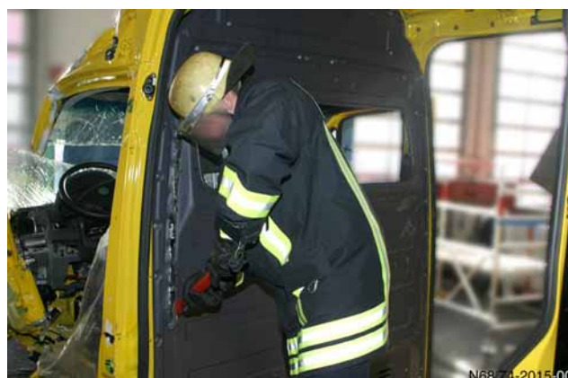
Cutting open the partition wall using a hooligan tool
