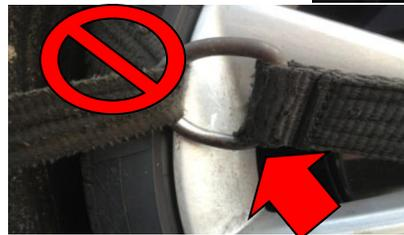
The example to the right demonstrates a **WRONG** way of strapping; in this case, the wheel was damaged due to metal-on-metal contact (red arrows).
